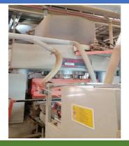
State of art presses with high pressing capacity from Sacmi & SITI
