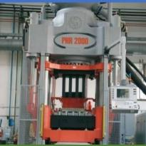
State of art presses with high pressing capacity from Sacmi & SITI
